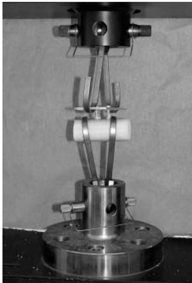
Figure 1. The axial pull-out of the plates applied to Synbone osteoporotic bone model with two locking screws.
