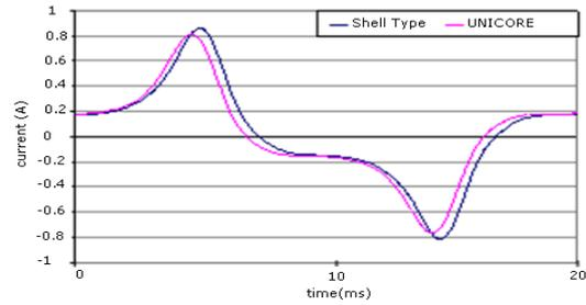
**Figure 3.** No-load currents of CWC and UNICORE transformers [22].
