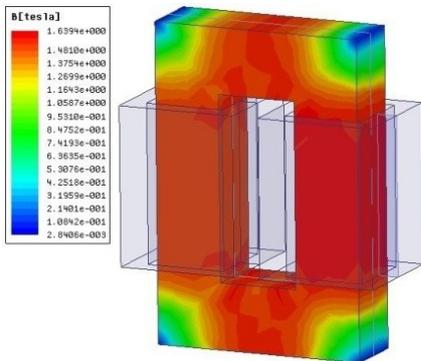
**Figure 2. (a)** Shell-type single phase transformer core analysis
