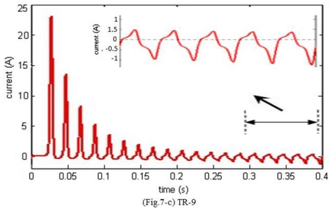
**Figure 9.** Inrush currents of the transformers-7-8-9.
