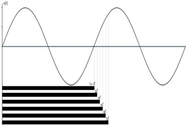
**Figure 5.** The transformer energization points of sine wave
