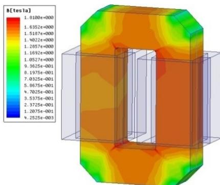
**Figure 2. (b)** UNICORE single phase transformer core analysis.
