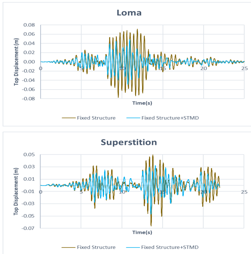
Figure 4 Top displacement time history of fixed base structure responses with and without STMD under Superstition and Loma record motions.
