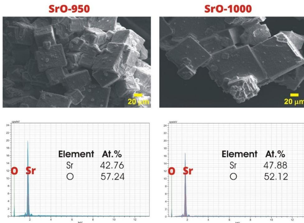
**Fig. 3.** Morphological analysis of both SrO samples
