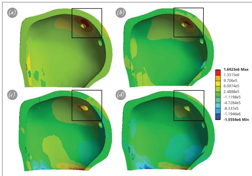
**Fig. 4.** Maximum shear stress of screw-bone interface: **(a)** Model A; 1.69 MPa, **(b)** Model B; 1.41 MPa, **(c)** Model C; 1.29 MPa, and **(d)** Model D; 0.75 MPa. [Color figure can be viewed in the online issue, which is available at [www.aott.org.tr](http://www.aott.org.tr)]
