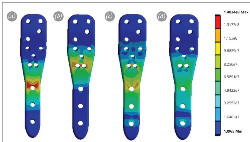
**Fig. 5.** Maximum von Mises stresses of the locking plate. **(a)** Model A; 148.24 MPa, **(b)** Model B; 132.01 MPa, **(c)** Model C; 116.83 MPa, and **(d)** Model D; 68.58 MPa. [Color figure can be viewed in the online issue, which is available at [www.aott.org.tr](http://www.aott.org.tr)]
