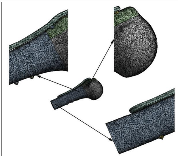
**Fig. 2.** Illustration of analysis model after meshing with Solid 187 element. [Color figure can be viewed in the online issue, which is available at [www.aott.org.tr](http://www.aott.org.tr)]
