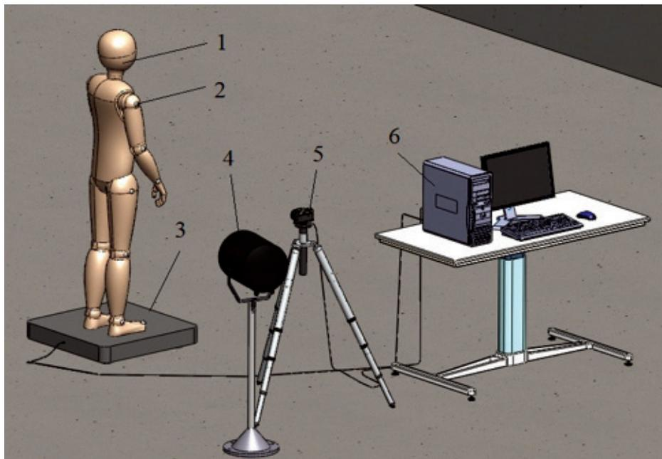
**Fig. 3.** CAD presentation of the analysis process. 1: The subject; 2: Markers; 3: Force platform; 4: Light; 5: Digital video camera; 6: Computer. [Color figure can be viewed in the online issue, which is available at [www.aott.org.tr](http://www.aott.org.tr)]
