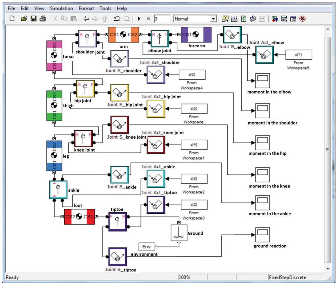
Fig. 2. SimMechanics™ block diagram of the link-segment model. [Color figure can be viewed in the online issue, which is available at [www.aott.org.tr](http://www.aott.org.tr)]
