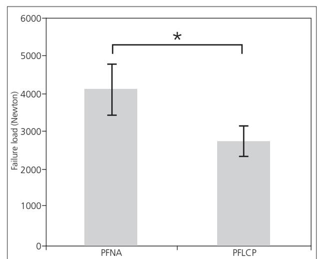
**Fig. 2.** Comparison of failure loads between the PFLCP and PFNA groups (Newton). \*Significantly different.
