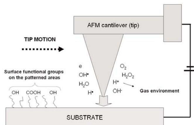
Figure 2. Schematic description of c-AFM nanolithography.
