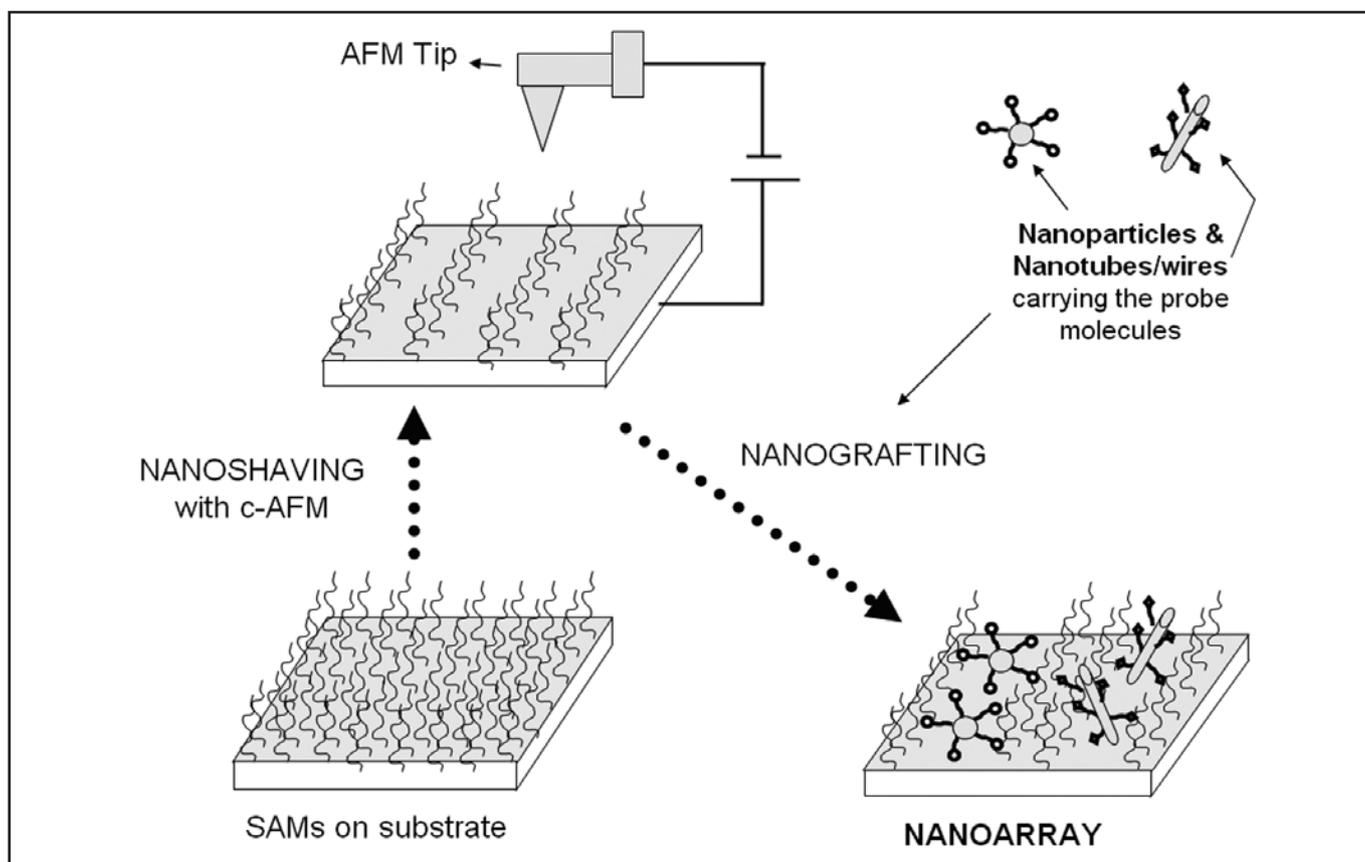
Figure 4. Schematic description of nanografting.
