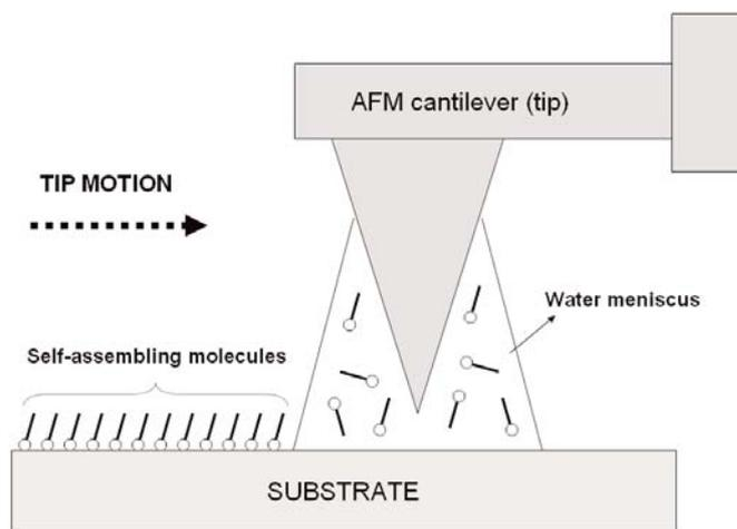
Figure 1. Schematic description of the dip-pen nanolithography.
