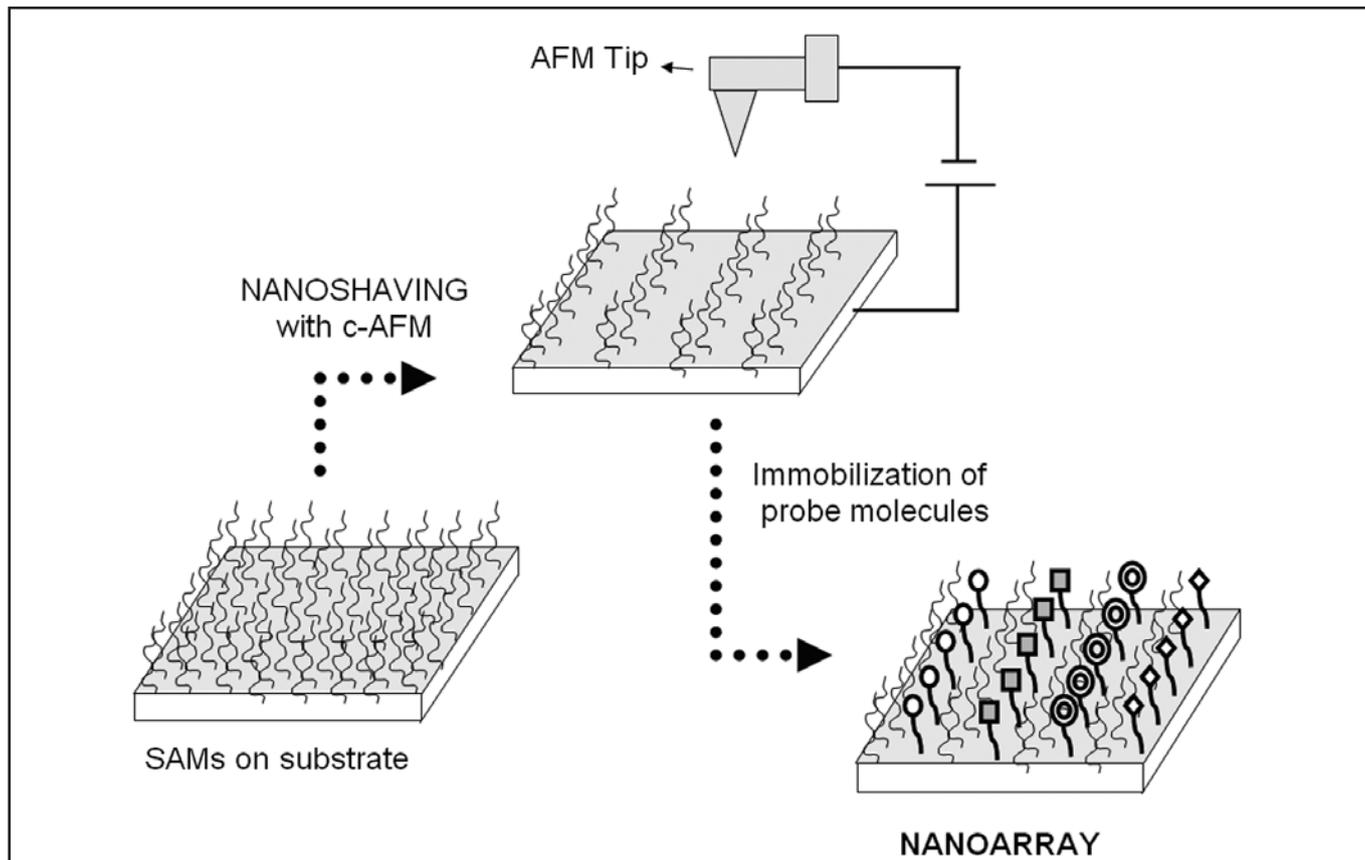
Figure 3. Schematic description of nanoshaving.
