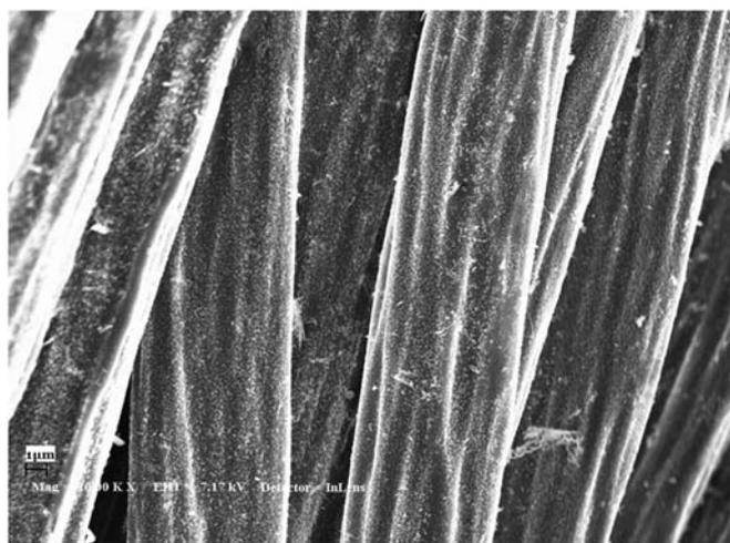
Figure 3. SEM micrographs of carbon fibers after chemical activation, before aluminum deposition was washed with nitric acid treatment. Magnification = 10.00 KX.
