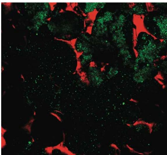
**Figure 4.** A confocal microscopy image of the scaffold. Interconnectivity is clearly seen from the image. Please note that these scaffolds were incorporated a pigment (Solvent Green 3) for better visualization of the pore morphology.
