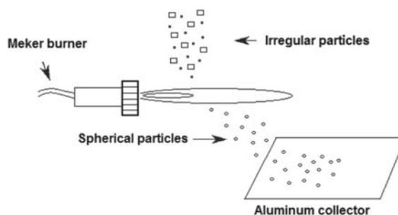
**Figure 1.** Schematic illustration of the spherical sugar particles production by flame.
