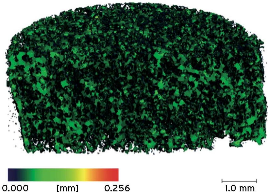
**Figure 3.** Micro-CT image of the scaffold prepared by spheroidized sugar porogen.
