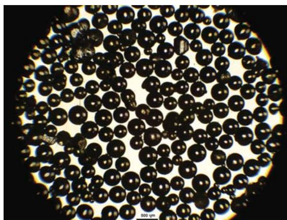
**Figure 2.** Optical micrograph of the spheroidized sugar particles (sieved, 250-355  $\mu$ m).
