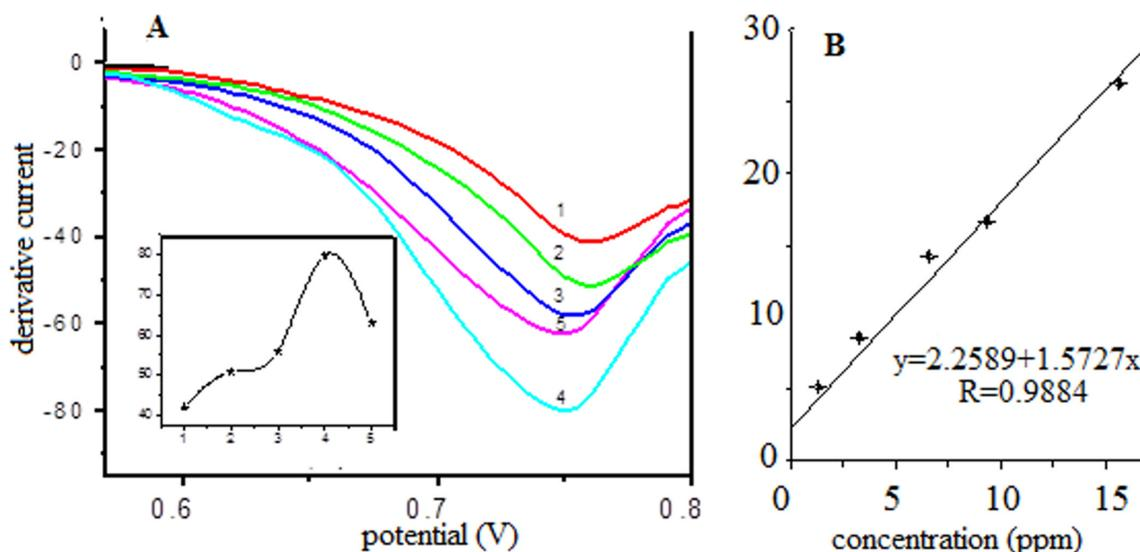
**Figure 3.** A) Derived voltammograms of MCPE electrode prepared with different particles size of graphite powder (1) 0.5-0.2 mm; (2) 0.2-0.16 mm; (3) 0.16-0.09 mm; (4) 0.09-0.071 mm; (5) 0.071-0.056 mm, with phenol concentration 3.3 ppm, in phosphate buffer 0.1M (pH 7), scan rate 50 mV/s, B) Calibration curve obtained at potential 0.78 V for 0.09-0.071 mm granulometry.
