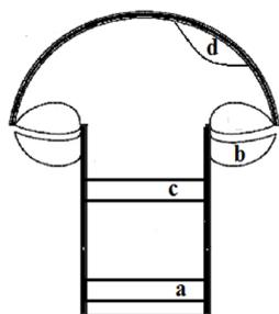
**Figure 1.** Different part of mushroom used as sensor modifier: a) bottom of stem, b) gill, c) upper of stem, d) cap.
