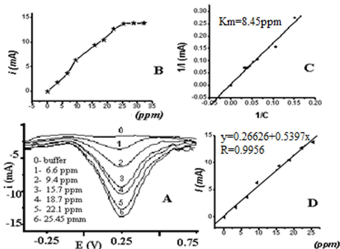
**Figure 5.** A) Voltammograms of MCPE obtained in different catechol concentration (pH 7.0). B) Current obtained vs. catechol concentration. C) The regression of the sensing experimental data by Michaelis-Menten model. D) Sensor calibration in linear zone.
