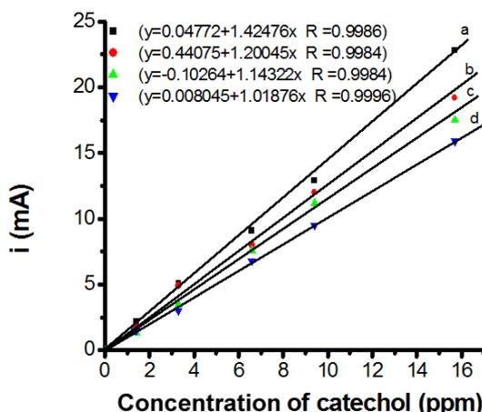
**Figure 4.** Calibration curves of CPEM using a.b.c.d section as modifier,  $E = 0.4 \text{ V}$ , scan rate  $50 \text{ mV/s}$ .
