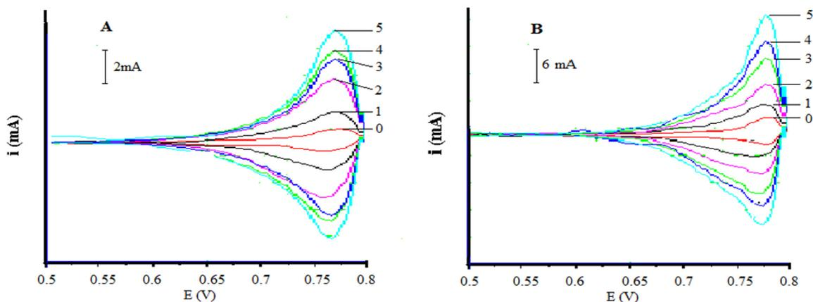
**Figure 2.** Cyclic voltammograms in 0.1 M phosphate buffer pH 7, scan rate = 50 mV/s. using CPE (A) and MCPE (B), in different phenol concentrations (0) buffer, (1) 1.4 ppm, (2) 3.3 ppm; (3) 6.6 ppm; (4) 9.4 ppm; (5) 9.4 ppm; using CPEM in the same phenol concentrations.
