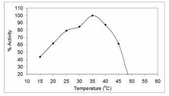
Figure 6. Optimal temperature for brain AChE.
