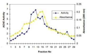
Figure 1. Purification of liver homogenate AChE by affinity chromatography the columns  $(1.3 \times 60 \text{ cm})$  eluted by buffer C at pH 8. It was buffer at 20 ml/h flow rate for fraction volumes of 6 ml.
