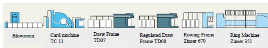
**Figure 1.** Ring spinning production line
