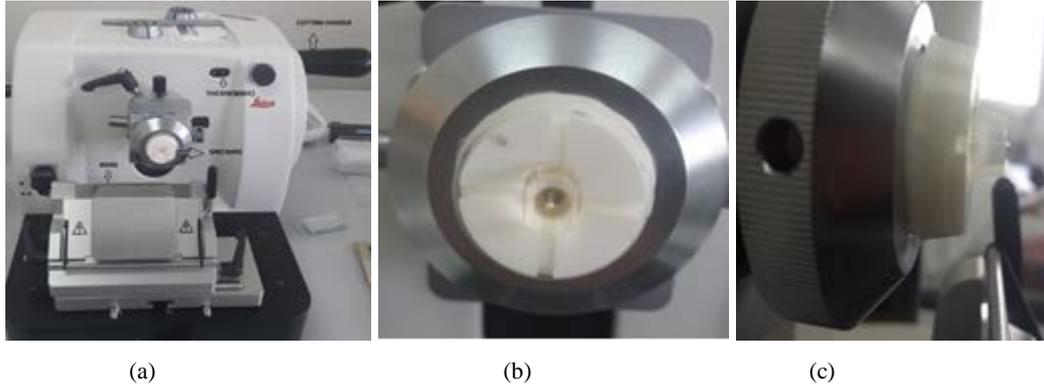
**Figure 3.** Microtome and yarn sample mold views; (a) Microtome (b) yarn sample mold front view (c) yarn sample mold side view
