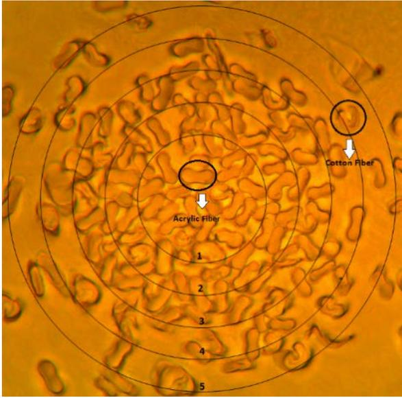
Figure 2. Dividing the yarn cross-section into 5 equal areas
