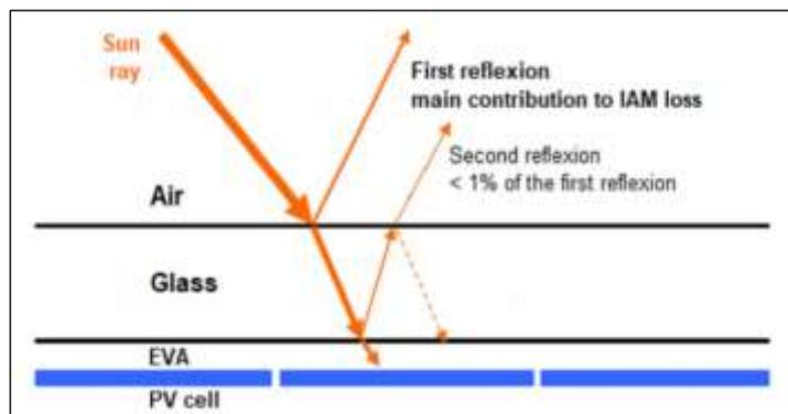
Figure 2. Array incidence loss
