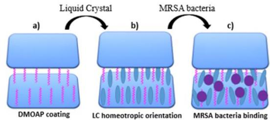
**Figure 1.** Detection principle of LC-based sensing procedure: a) coating of glass slides with DMOAP alignment agent, b) assembling of the LC molecules on the DMOAP coated glass slide, c) binding of MRSA bacteria to DMOAP-coated surface.
