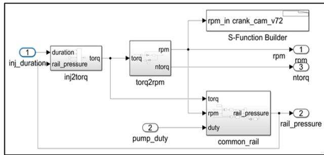
Figure 2. Engine model
