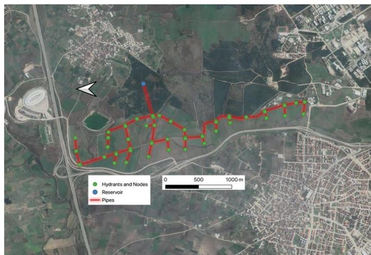
**Figure 3- The layout of Yolcati pressurized irrigation network**
