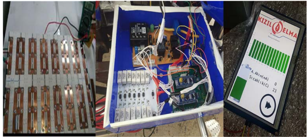
Figure A. Braiding battery package and the proposed passive balancing-based battery management system (BMS)
