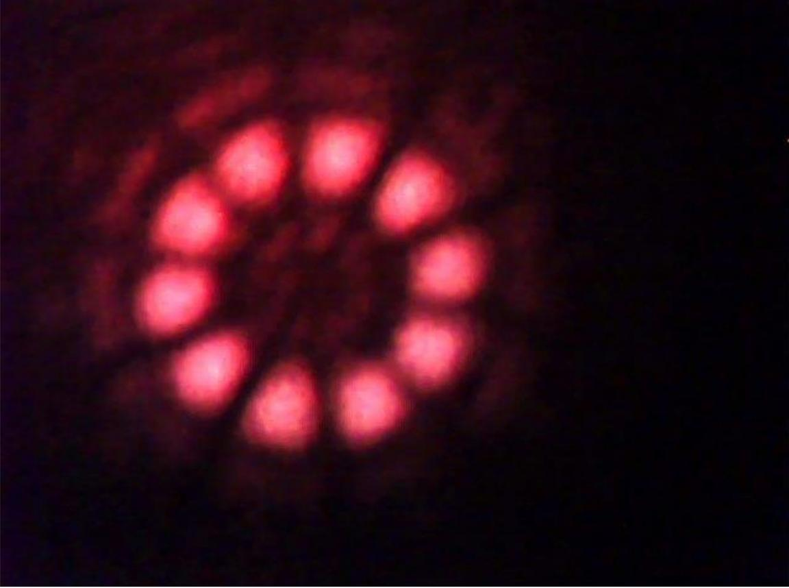
**Figure 6.** The intensity patterns of two counter-propagating twisted light
