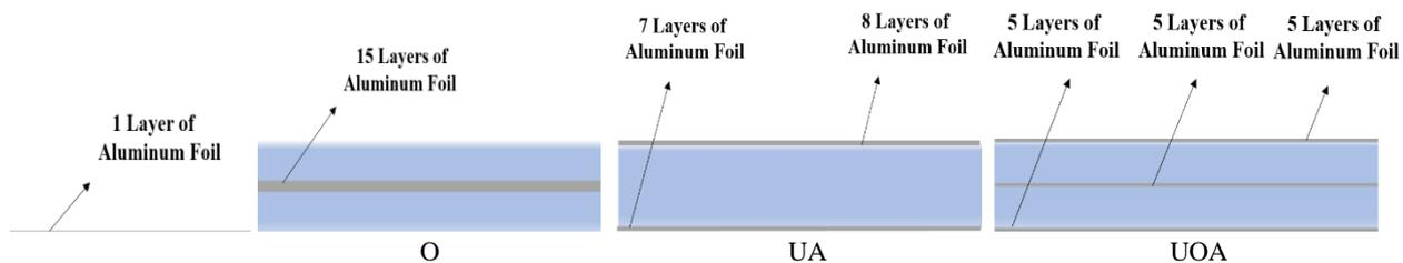
Figure 3. The Layout of Aluminum Surface/s In samples
