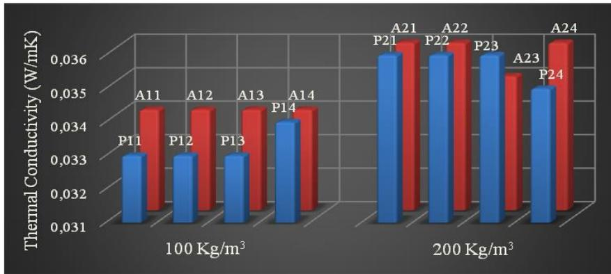
Figure 6. The effect of fiber difference on thermal conductivity coefficient
