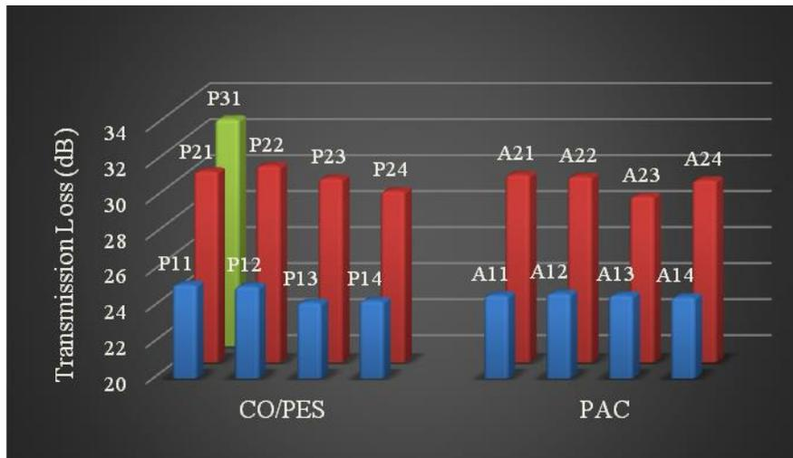
**Figure 8.** Effect of density change on sound transmission loss
