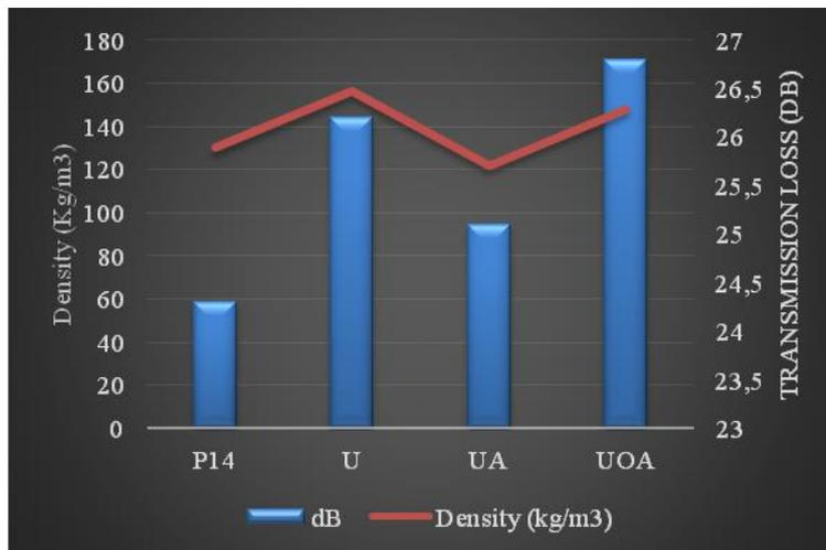
Figure 11. Comparative sound transmission loss values
