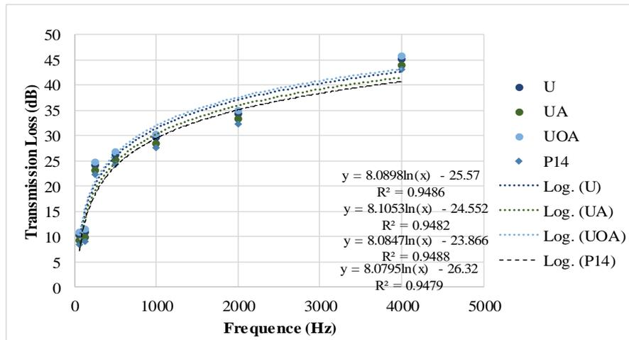
Figure 12. Comparative sound transmission loss values
