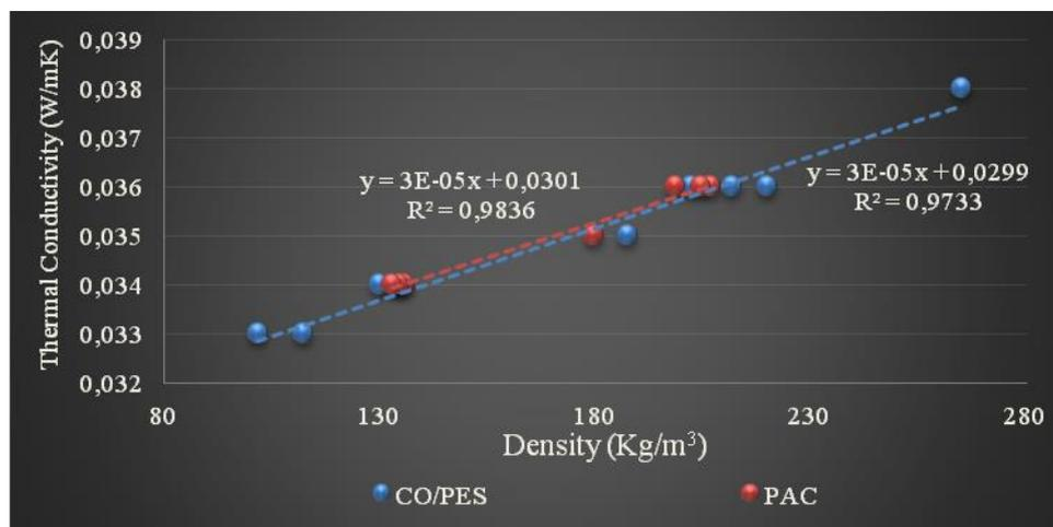
Figure 5. The correlation between density and thermal conductivity coefficient
