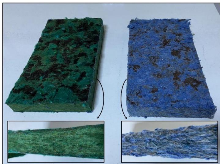
**Figure 2.** View of two samples of produced acrylic and cotton/polyester panels
