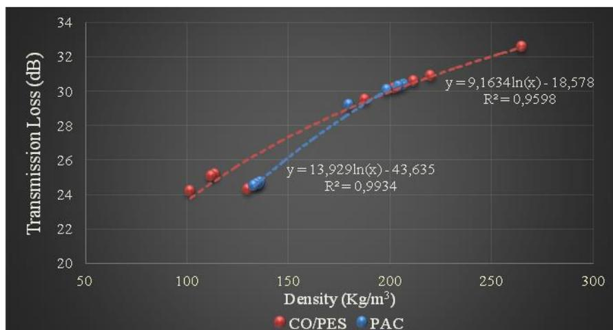
**Figure 9.** The correlation between density change and sound transmission loss
