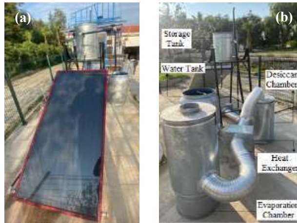
Figure 2. Photographs of the designed SD-SDAEC system (a) front view and (b) rear view
