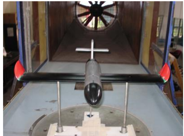
Fig. 17. Airplane model with winglet in wing tunnel
