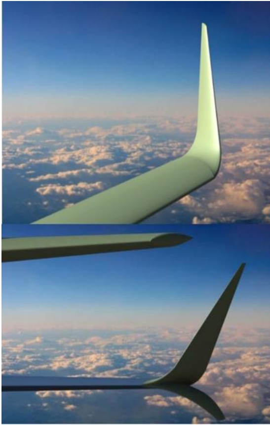
Fig. 7. Blended winglet on top, maxi winglet on bottom [12]
