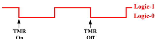
Fig. 11. The use of Timer in detecting the period and frequency
