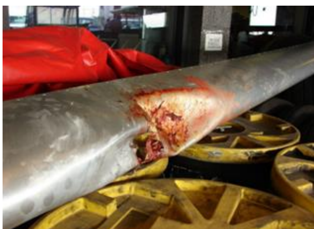
Fig. 2. Bird strike damage to B737 aircraft left wing leading edge [3]
