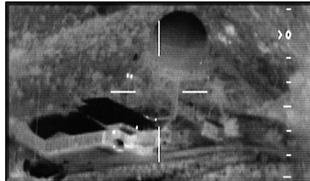
Figure 25. FLIR Can Not Detect Light Sources Unless Thermally Significant.
