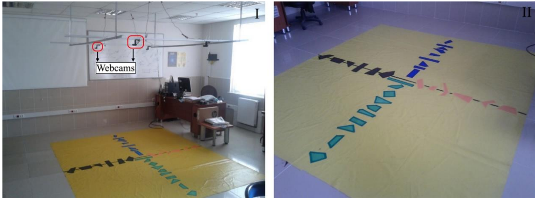
Figure 11 (I) Multi-camera configured real operating environment (II) Colored and randomly shaped labels on the operating floor
