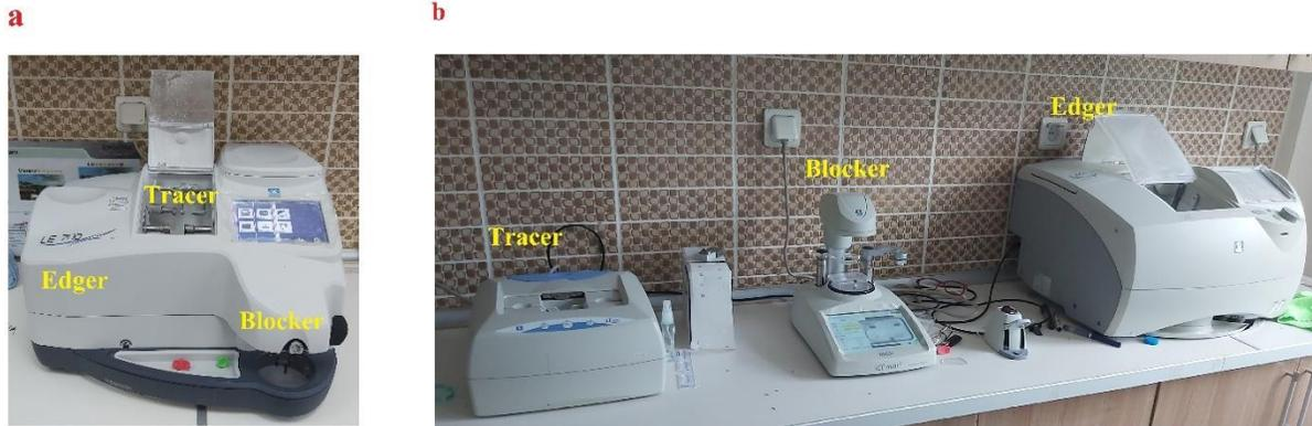
**Figure 8.** Figure illustrates edgers with internal tracer and blocker (a) and edger with external tracer and blocker (b).
