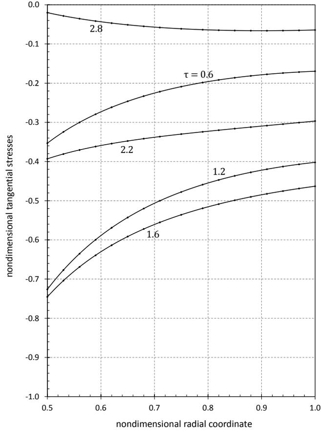
FIGURE 4. Nondimensional tangential stress. Solid lines denote the analytical solution, while dots indicate the numerical results.  $q = 0.15$ .
