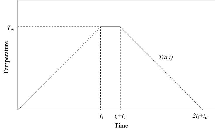
FIGURE 1. Periodic boundary condition applied to the inner surface of the tube.
