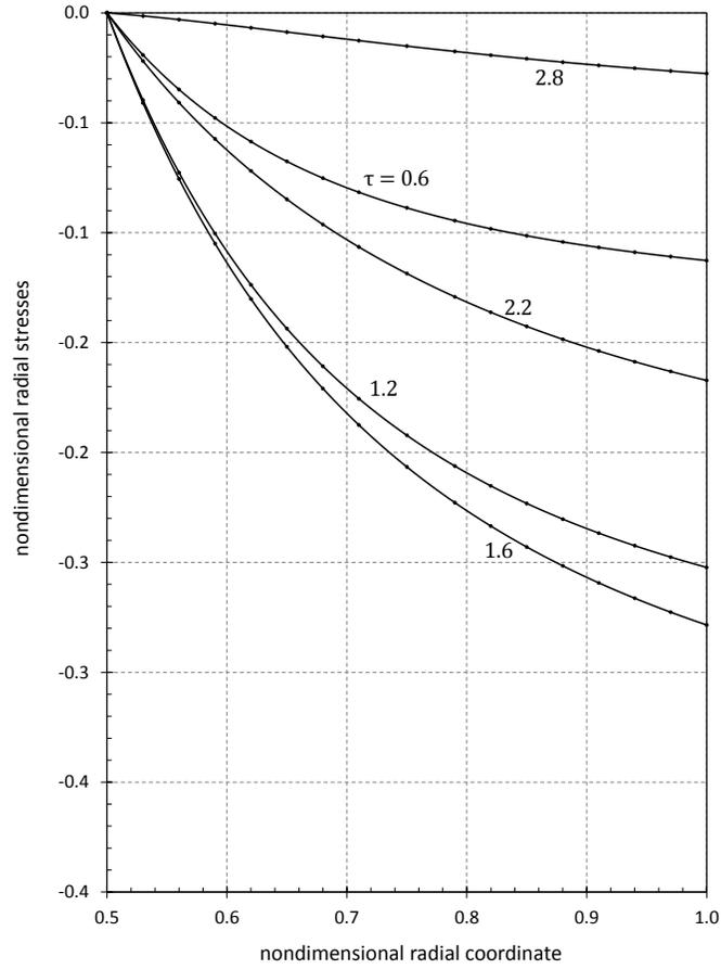
FIGURE 3. Nondimensional radial stress. Solid lines denote the analytical solution, while dots indicate the numerical results.  $q = 0.15$ .
