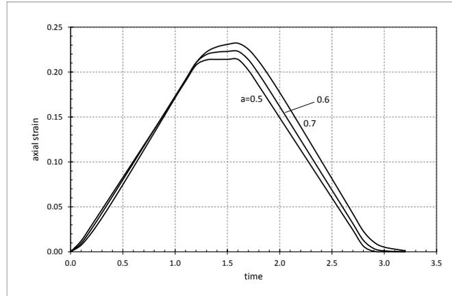
FIGURE 6. Evolution of the axial strain for different values of the inner radius during periodic heating.  $q = 0.15$ .
