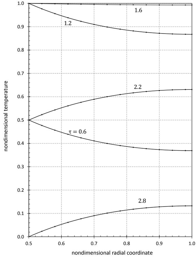
FIGURE 2. Temperature distribution in the tube at different time steps. Solid line denotes the analytical solution, while dots indicate the numerical. The parameters are used:  $\tau_t = 1.2$  and  $\tau_c = 0.4$ .
