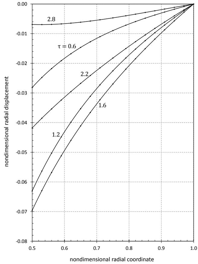
FIGURE 5. Nondimensional radial displacement. Solid lines denote the analytical solution, while dots indicate the numerical results.  $q = 0.15$ .
