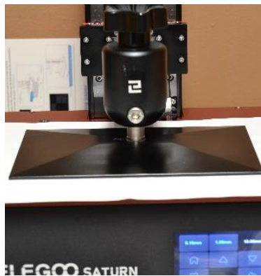
Figure 7. Using a plain A4 paper between the LCD and the build platform.
