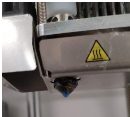
Figure 5. Molten plastic leaking from top of the heat block.
