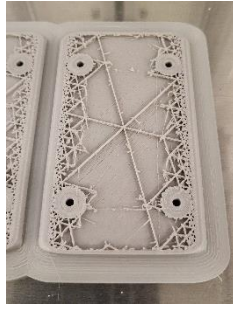
Figure 2. 3D print with incomplete filling.
