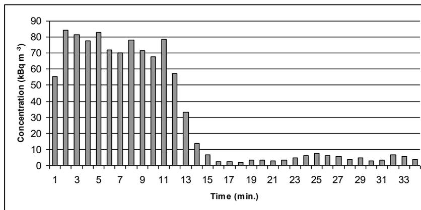
**Figure 3.** Representative results in the soil gas measured using the AlphaGuard monitor (from B12 district)
