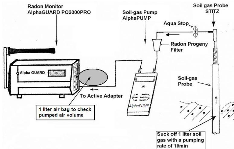
**Figure 2.** Schematic set-up of AlphaGUARD radon-thoron monitoring in the soil gas.
