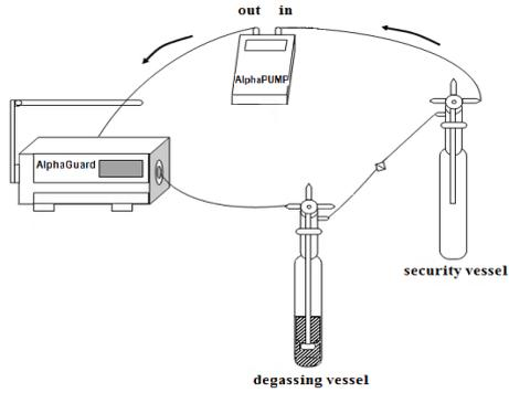
**Figure 4.** Schematic view of the AquaKIT measuring set-up in water
