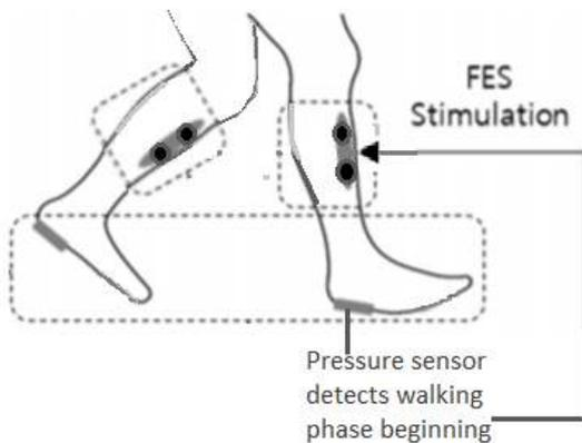
Figure 5. Schematic of the FES control algorithm
