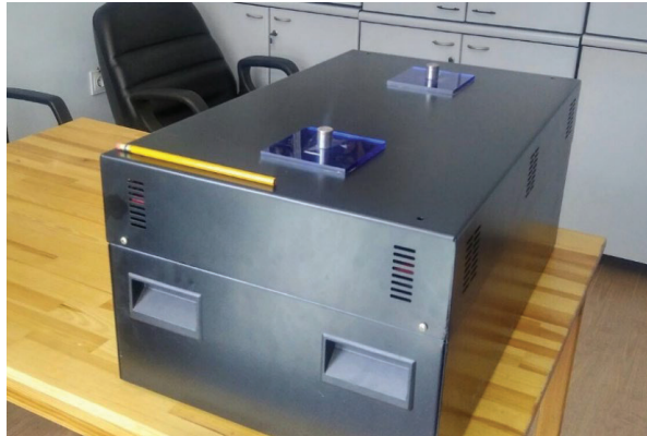
Figure 3 An experimental battery pack of 24V, 7kWh with analog BMS
