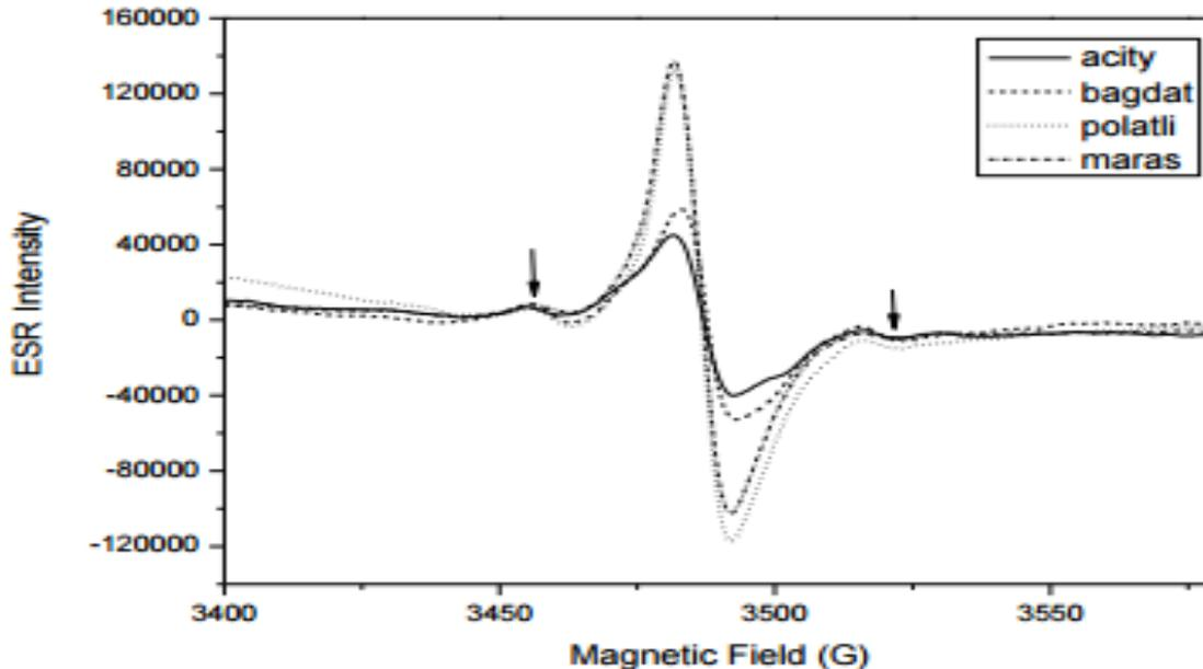
**Figure 3:** Results of ESR measurements at the end of six month for red peppers from all origins (Arrows represent radiation induced cellulose peaks and magnetic field difference between peaks is nearly 60 Gauss)
