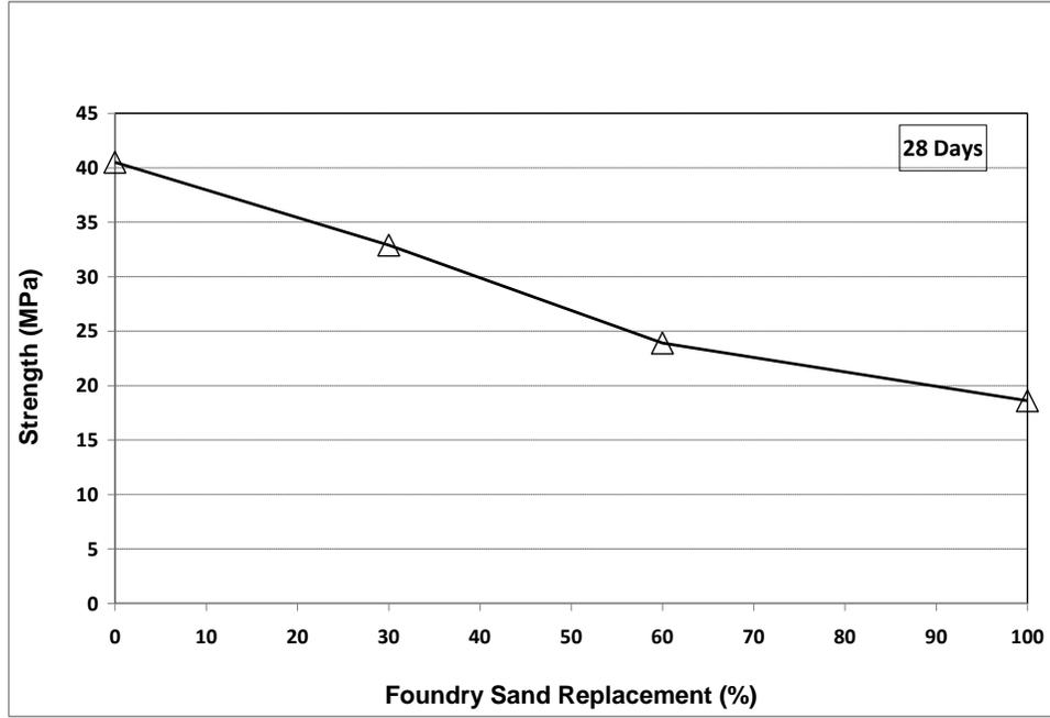
Figure 4. Compressive strength of concretes containing varying amounts of foundry sand at 28 days of curing
