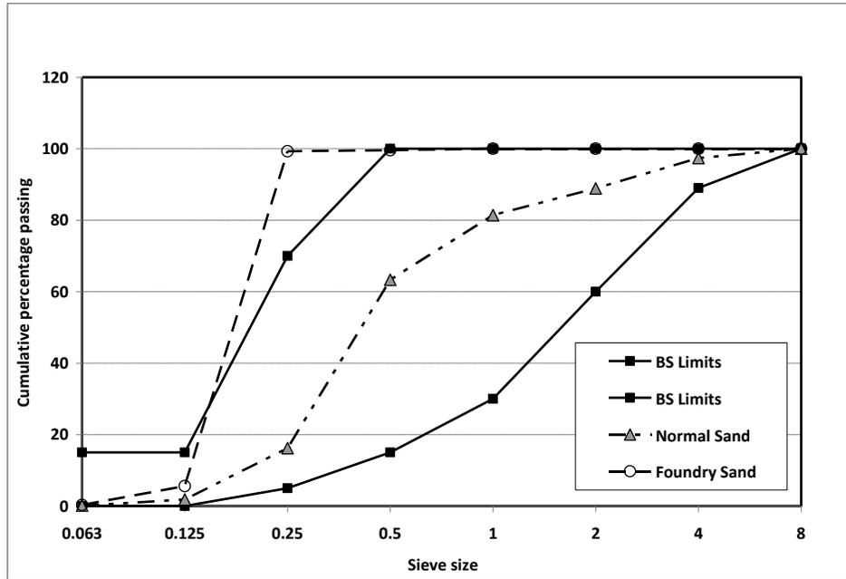
Figure 1. Particle size distribution of normal sand and foundry sand
