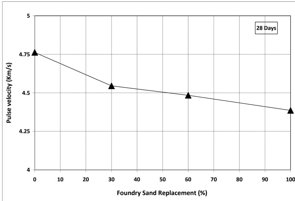
Figure 5. Ultrasonic pulse velocity (UPV) of concretes containing varying amounts of foundry sand at 28 days of curing
