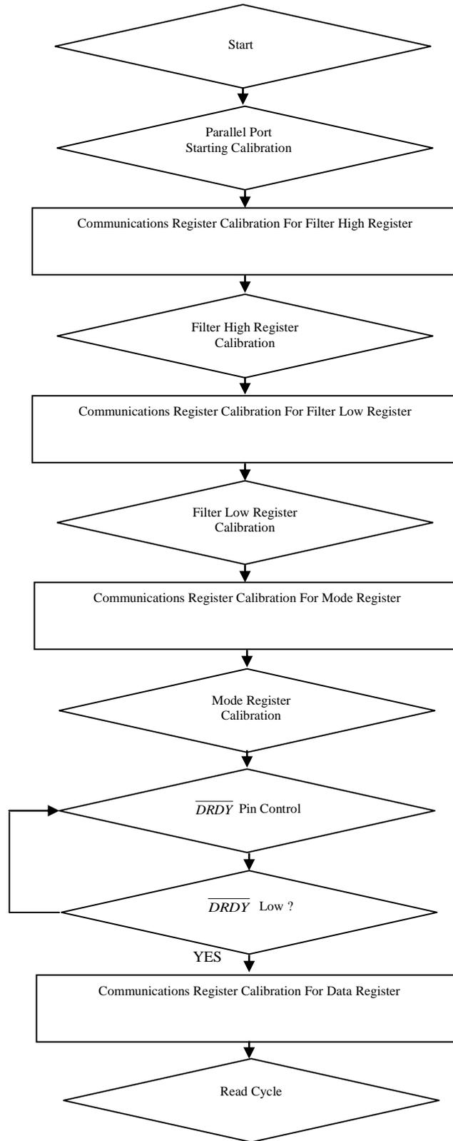
Figure 4. Flowchart for setting up and reading from the AD7714
