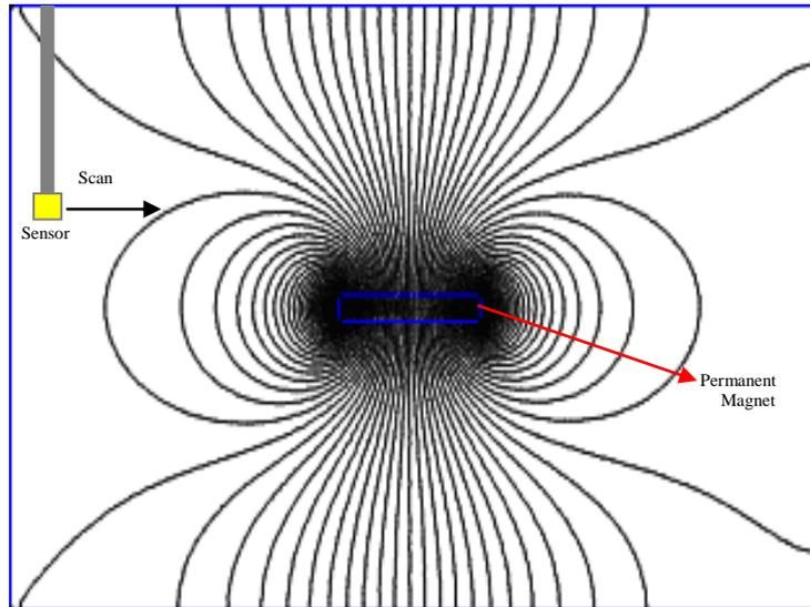
Figure 7. Magnetic flux variation at the sensor scanning axis
