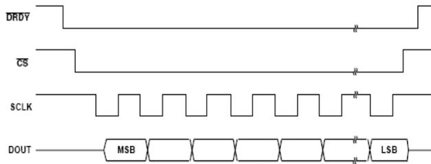
Figure 2. Read cycle timing diagram (POL=1)
