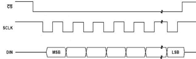
Figure 1. Write cycle timing diagram (POL=1)
