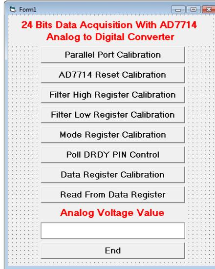
Figure 5. Programming interface for setting up and reading from the AD7714
