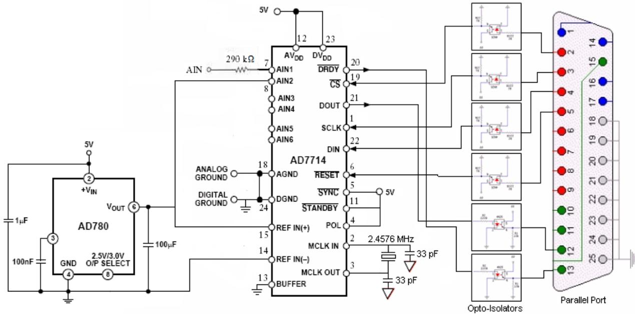
Figure 3. Data transfer from parallel port
