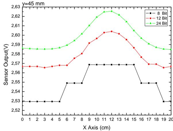
Figure 10. The sensor output voltage variations for different resolutions along the x-axis.
