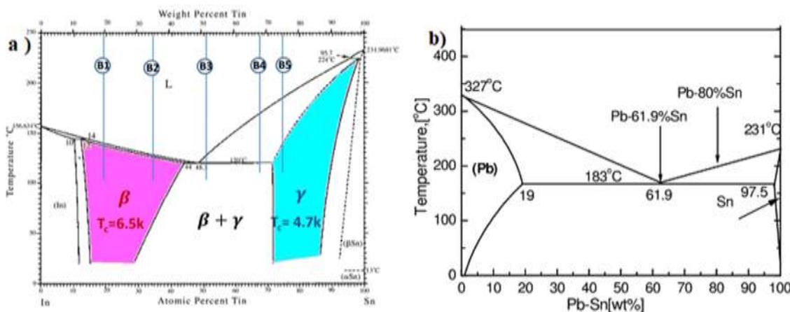
**Figure 1.** a) Phase diagram of binary SnIn [13] alloys and (b) Phase diagram of PbSn alloy [14].
