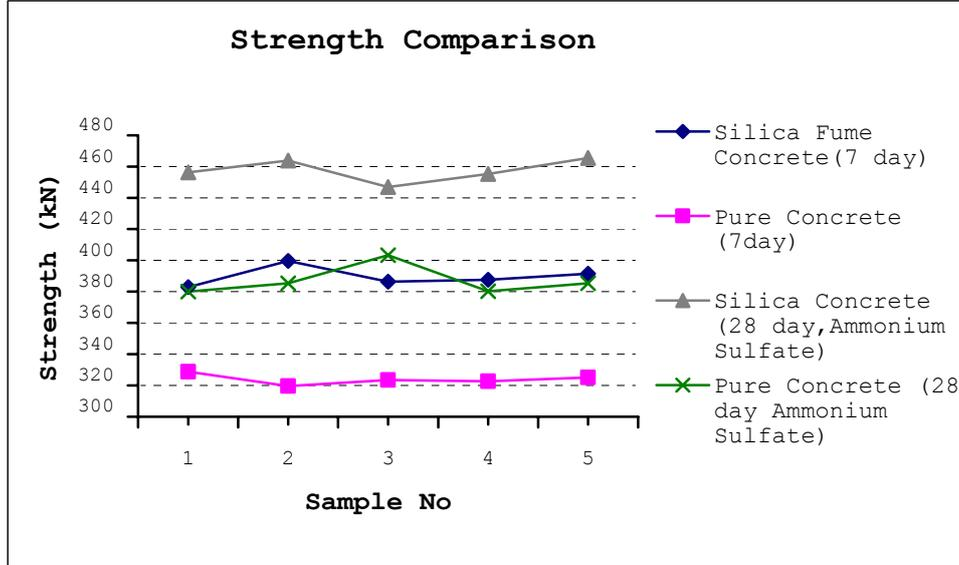
Figure 1. Comparison of 7-28 day strength of silica fume and pure concrete samples
