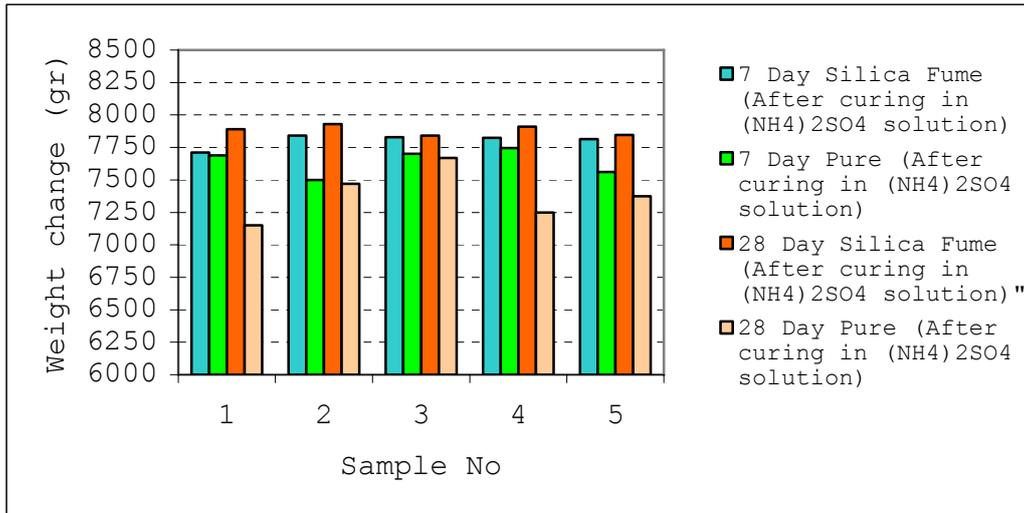
Figure 2. 7-28 day Weight change of silica fume and pure concrete samples
