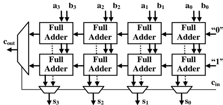
Figure 3. 4-bit carry select adder design
