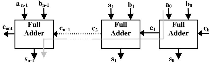
Figure 1.  $n$ -Bit generic ripple carry adder
