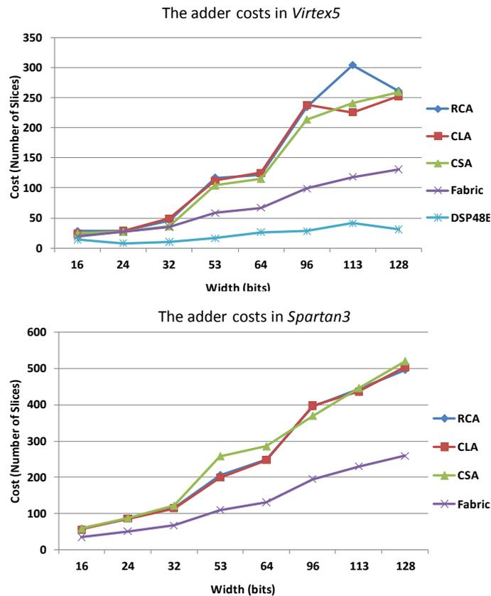
Figure 5. The comparison charts for costs of the adders in terms of slices on Virtex-5 and Spartan-3, respectively
