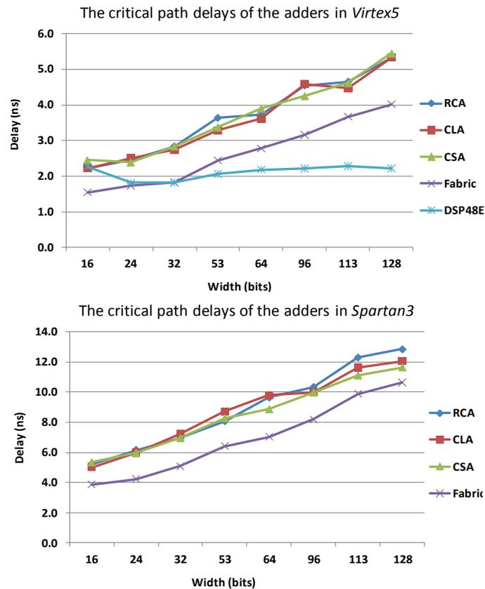
Figure 4. The comparison charts for critical path delays of the adders on Virtex-5 and Spartan-3, respectively.
