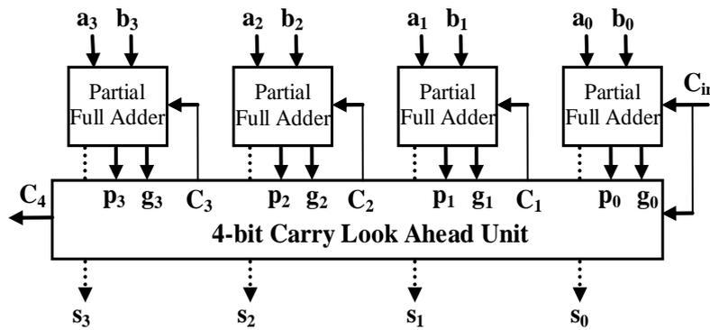
Figure 2. 4-bit CLA adder block diagram
