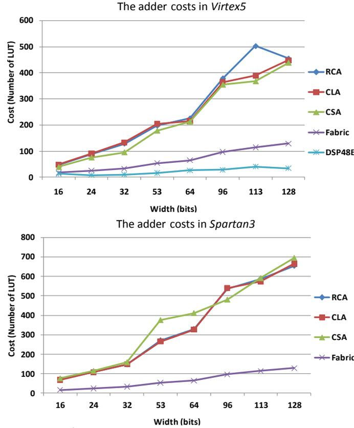
Figure 6. The comparison charts for costs of the adders in terms of LUTs on *Virtex-5* and *Spartan-3*, respectively
