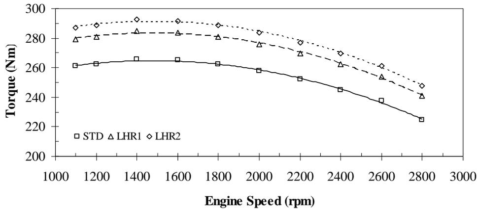
Figure 4. The variations of engine torque by engine speed for different insulation levels
