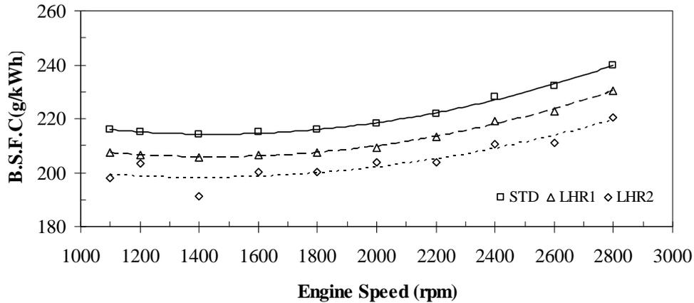
Figure 5. The variations of bsfc by engine speed for different insulation levels
