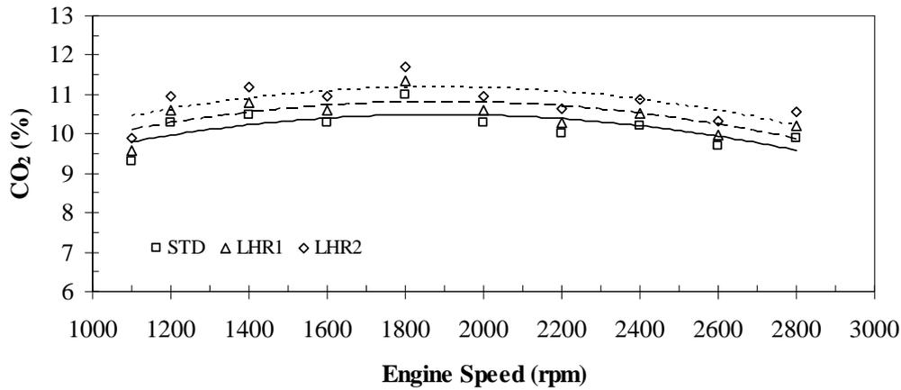
Figure 10. The variations of CO<sub>2</sub> emission by engine speed for different insulation levels
