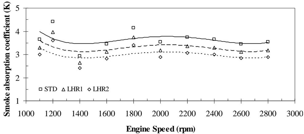
Figure 9. The variations of smoke emission by engine speed for different insulation levels
