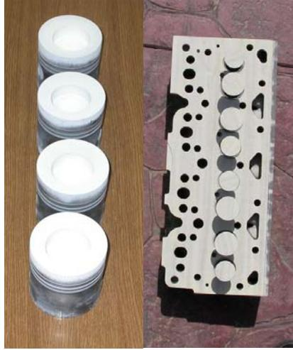
Figure 2. Ceramic coated parts of the test engine
