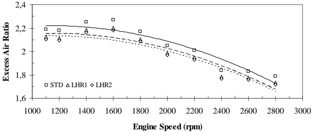
Figure 7. The variations of excess air ratio by engine speed for different insulation levels
