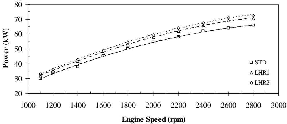
Figure 3. The variations of engine power by engine speed for different insulation levels
