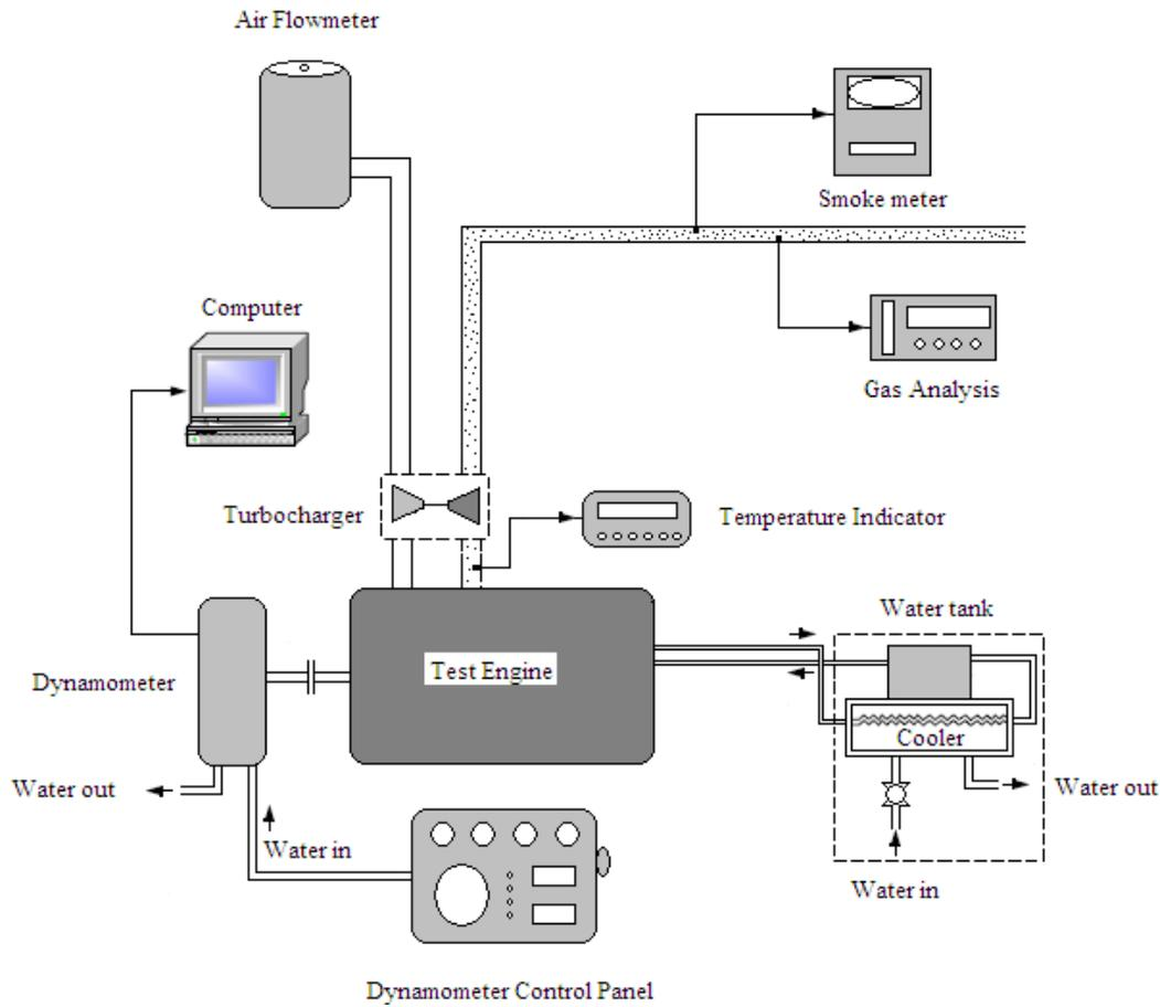
Figure 1. Schematic diagram of test set up
