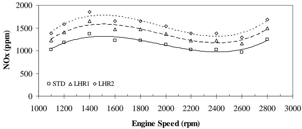
Figure 8. The variations of NO<sub>x</sub> emission by engine speed for different insulation levels
