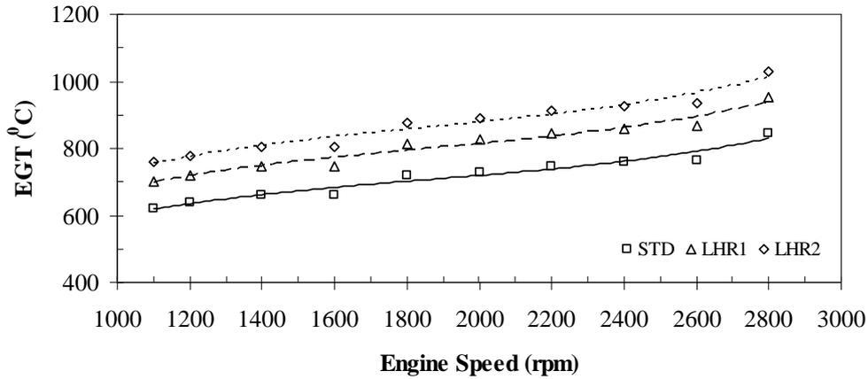
Figure 6. The variations of EGT by engine speed for different insulation levels
