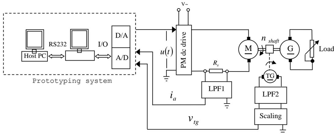
Figure 4. Schematic of laboratory setup
