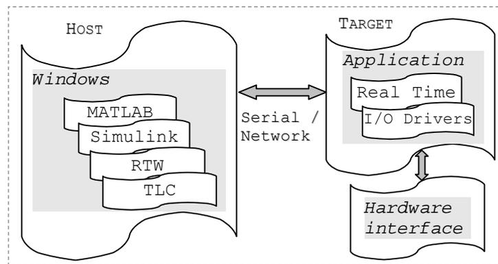
Figure 2. Host-Target real-time control system design
