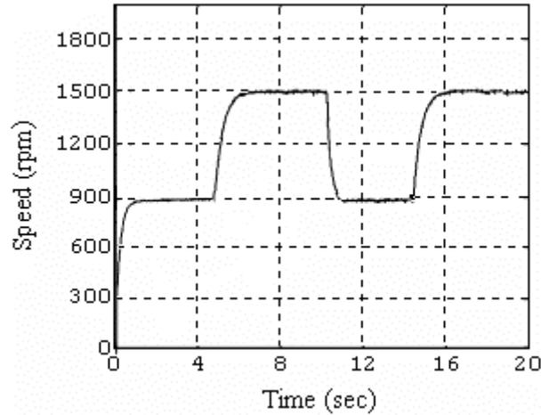
Figure 8. The OLC speed responses to the no load and full load disturbances at the reference of 1500 rpm
