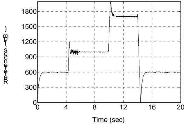
Figure 10. Speed responses of the CLC system to different reference speeds at full load
