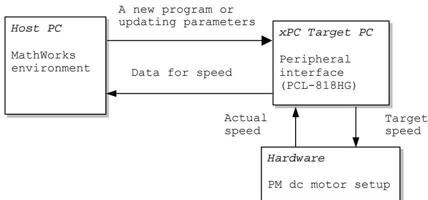
Figure 7. Flow diagram of the speed control system
