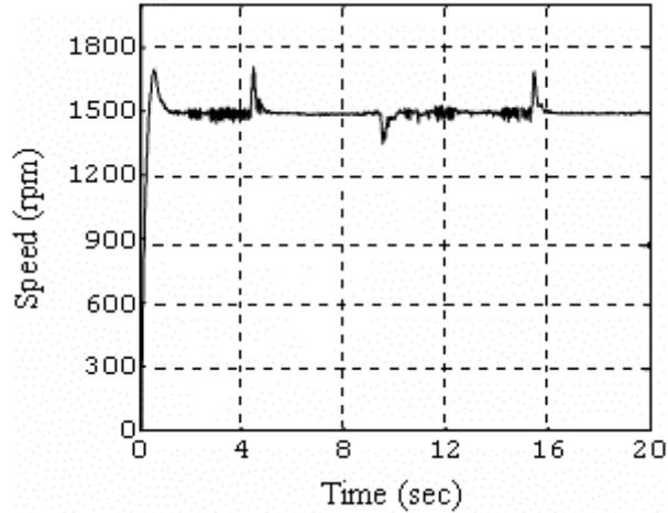
Figure 9. The CLC system speed responses to the no load and full load disturbances at the reference of 1500 rpm
