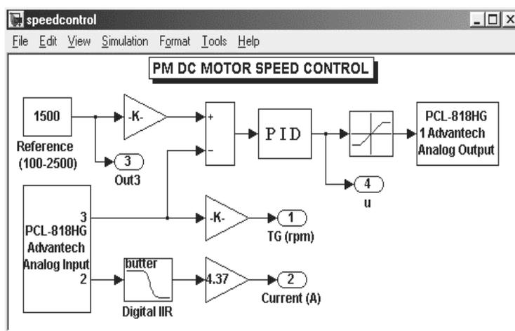
Figure 6. The real-time speed control of PM DC motor with Simulink
