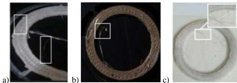
**Figure 3.** a) Test sample produced with ABS filament, b) Test sample produced with PLA filament c) Test sample produced with NYLON filament. (In the figure the lift-offs of the steel wire are shown).
