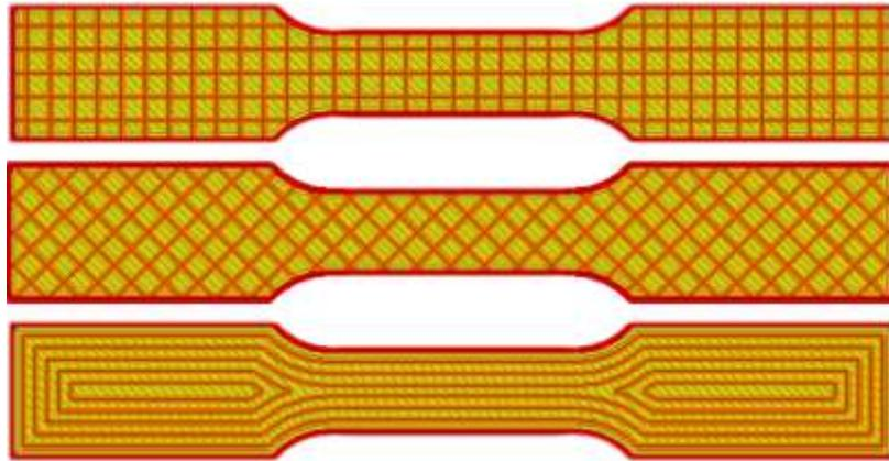
**Figure 5.** Grid, Crossed and Concentric patterns used in the production of samples.
