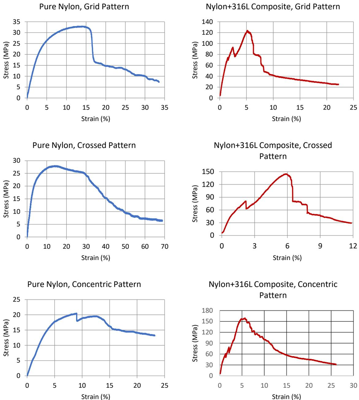
**Figure 6.** The graphics of tensile experiments of pure Nylon and Nylon + 316L Composite printings produced with three different pattern types.
