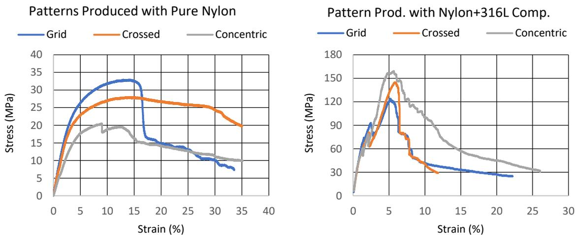
**Figure 8.** The comparative graphics of the Tensile experiments of 3 different pattern types produced with Pure Nylon and Nylon+316L Composite printings.
