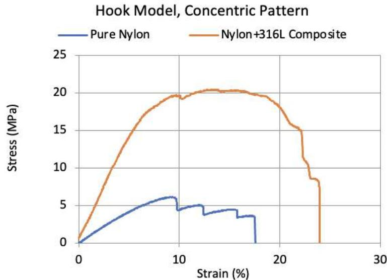
**Figure 10.** Tensile stress-strain curves of hooks.
