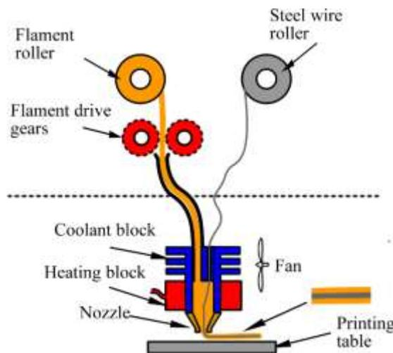
**Figure 2.** The Extruder mechanism developed for composite printing.
