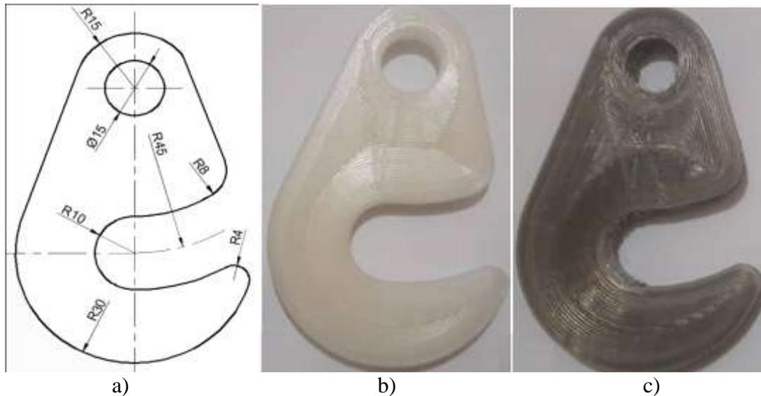
**Figure 9.** The real application model produced with concentric pattern. a) Dimensions, b) Pure Nylon model, c) Nylon+316L composite model.
