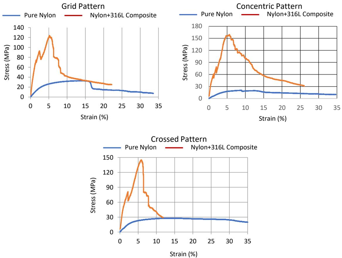
**Figure 7.** Comparative Tensile experiment graphics of three different pattern types produced with pure Nylon and Nylon+316L Composite printings.
