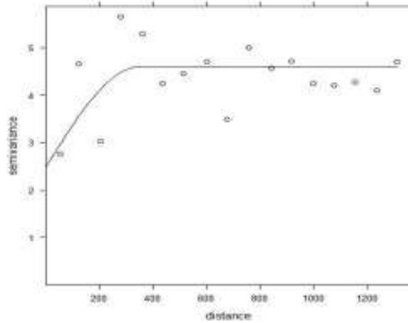
Figure 3. Variogram obtained by soil surface EC and Elevation in KED. (Nugget to sill ratio: 54 %, model: Spherical, range: 349)
