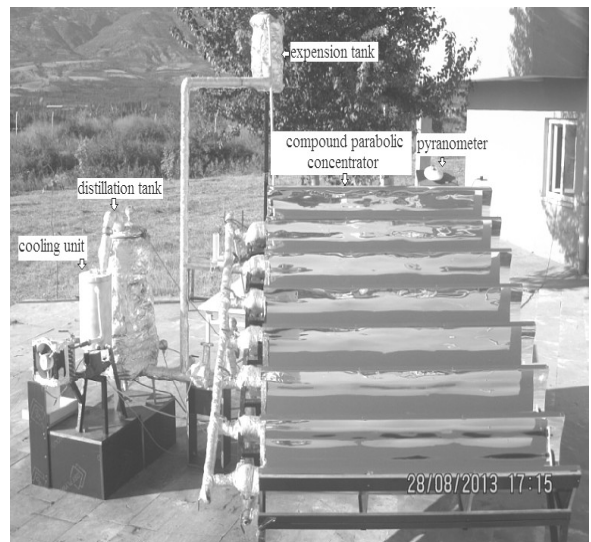
Figure 4. Assembled solar distillery with solar CPCs
