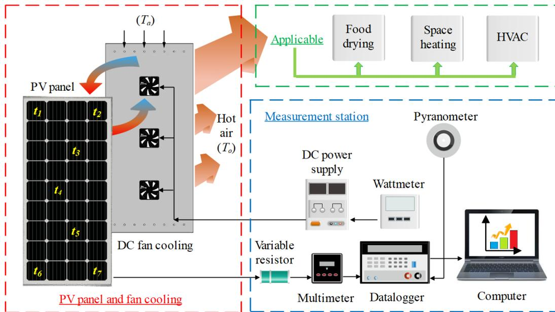
**Figure 2.** The schematic view of the experimental setup
