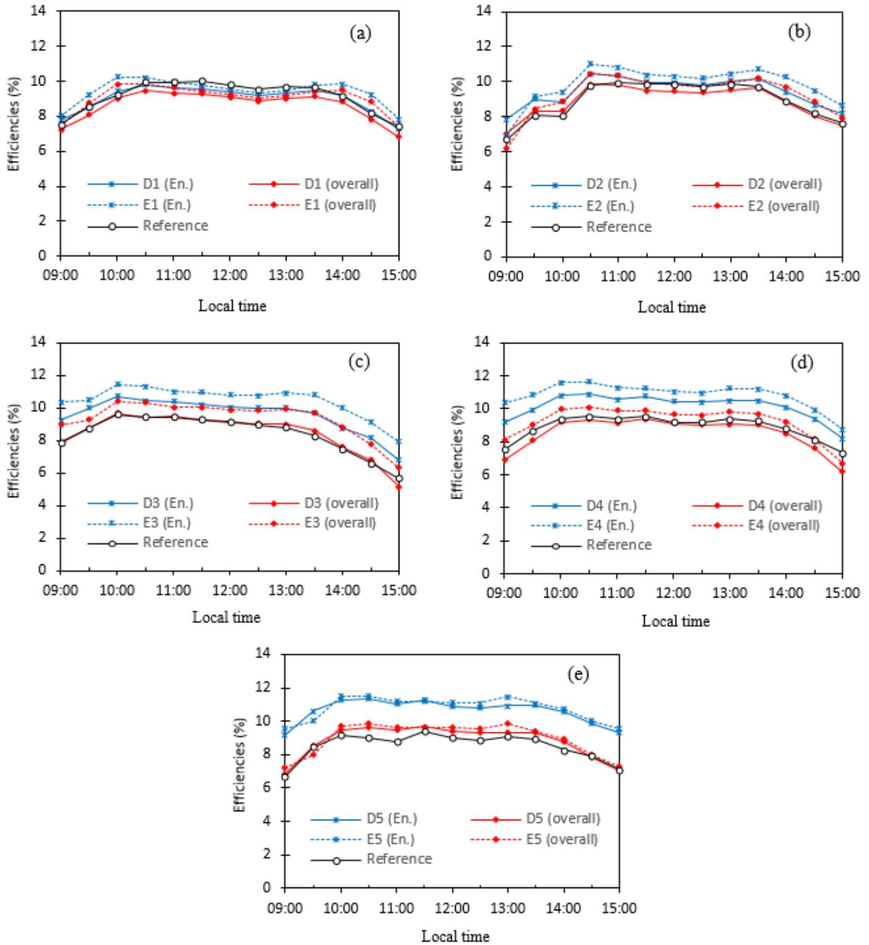
Figure 6. Efficiency values of PV panels with 3 and 4 DC fans
