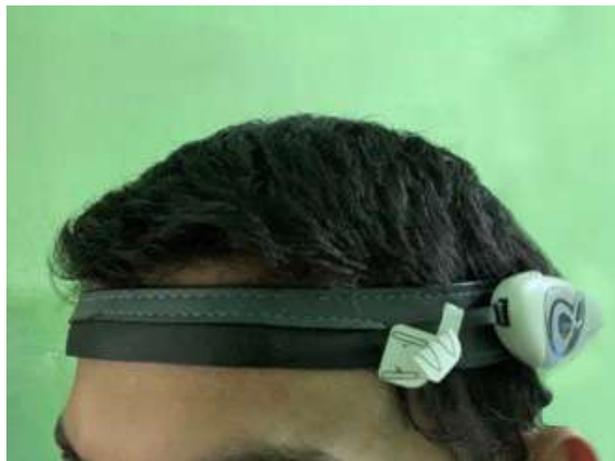
**Figure 8.** The headset is worn by making sure the metal nodes directly touch the forehead.
