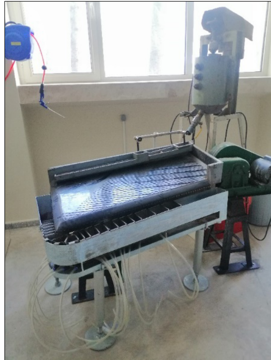
Figure 6. General view of shaking table with sand surface, feeder and sampling apparatus
