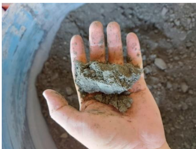
Figure 1 Consistency of RCC mixture
