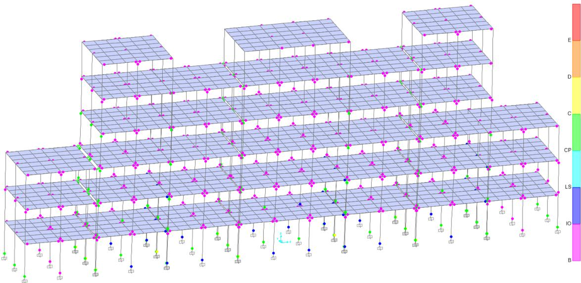
**Figure 3.** Plastic Hinges Graph for Joint Structures. Result of the Joint Conditions in case of the Strongest Earthquake (IO: Immediate Occupancy, LS: Life Safety, CP: Collapse Prevention, C: Collapse)
