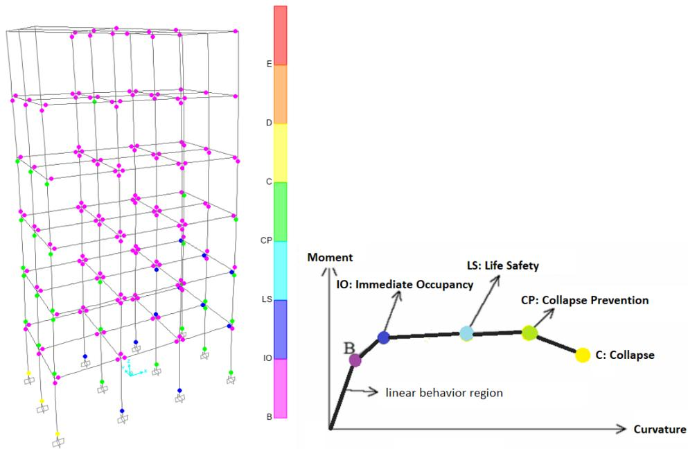
**Figure 4.** Plastic Hinges Graph for Single Structure Result of Analysis in case of the Strongest Earthquake.
