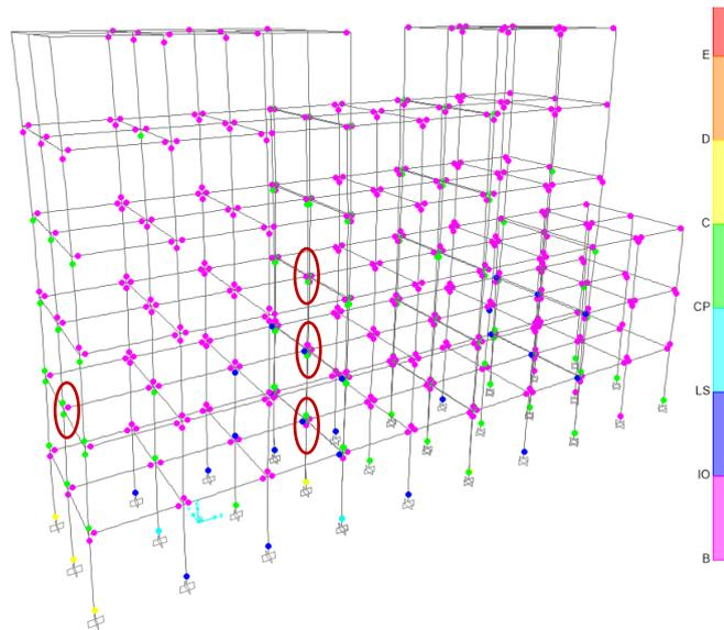
**Figure 6.** Plastic Hinge Graph for Structures that don't have Enough Adjacent Spans. Result of Analysis for the Strongest Earthquake.
