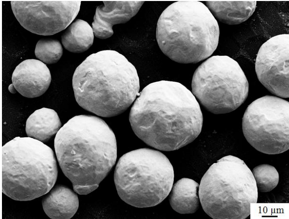
Figure 4: SEM micrograph of silver powder.
