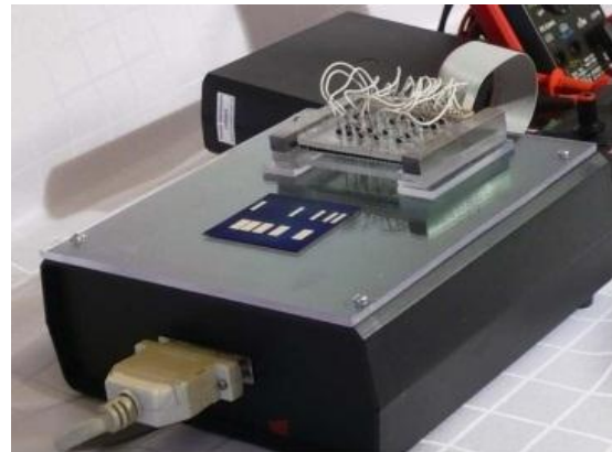
Figure 7: Measuring position of TLM method.
