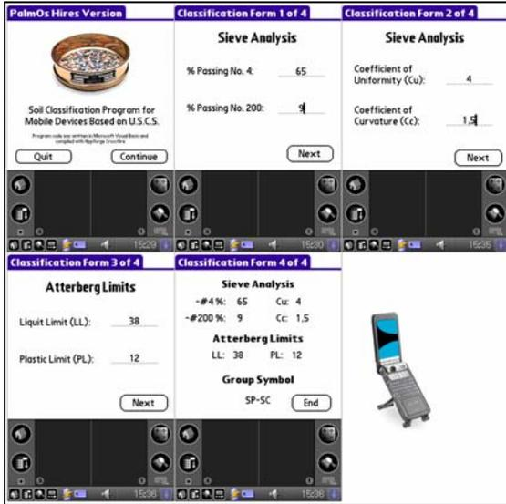
Figure 6. Visual Basic application on a Palm high resolution device.
