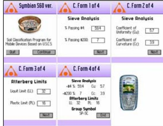
Figure 8. Visual Basic application on a Symbian 60 device.
