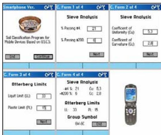
Figure 10. Visual Basic application on a Windows Mobile based Smartphone (Motorola Mpx 200).
